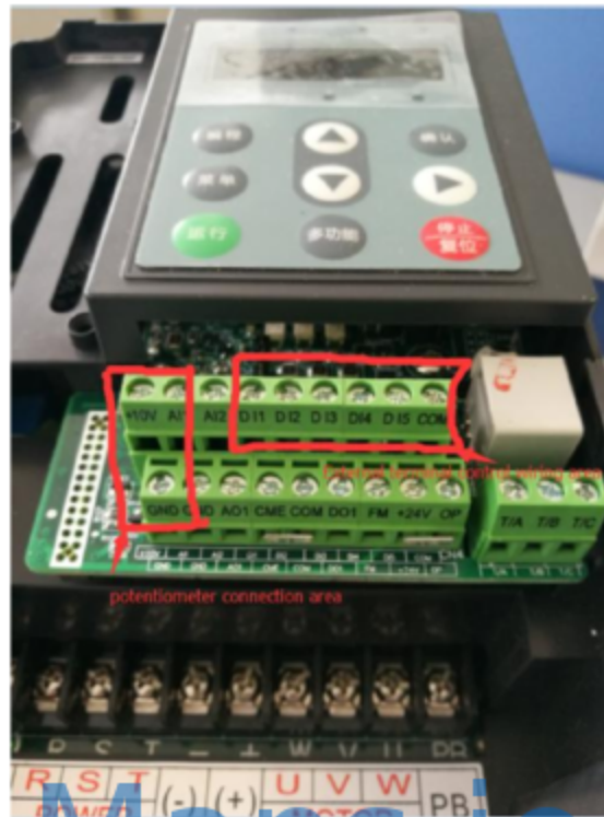
Fig.1 Open the front panel, find the analog input (10V, AI1, GND) and digital input terminals (DI1, DI2... DI5)
